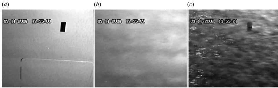
FIGURE 27. Images recorded during Test 2b of the roughened model surface at 6.8 \text{ m s}^{-1} : (a) no injection; (b) bubble drag reduction; and (c) air-layer drag reduction. The streamwise (right to left in images) and spanwise (top to bottom in images) directions of the model were observed by the recording system.
